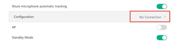
4.1 Click on "No Connection" to start the configuration, type the IP of the microphone in the red square and click on "Connect".
